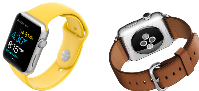
Figure 1. The Apple Watch, a smartwatch capable of tracking physical activity, heart rate, and location. The left photo shows the watch face, and the right photo shows the sensors for measuring heart rate. Photos by Wiyre Media.
